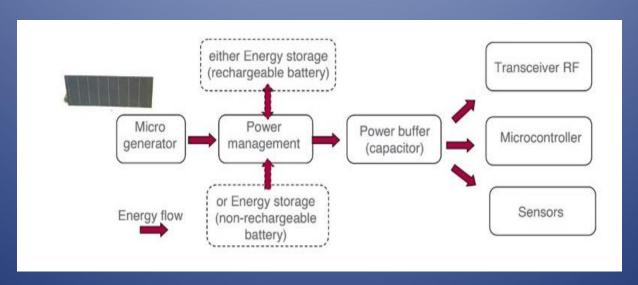
Typical Energy Requirements 1mJ per measurement Measurement frequency circa 10 to 50 per hour
